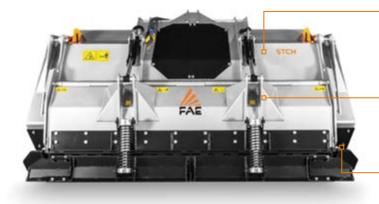
Hydraulic rear hood for an optimal material sizing and control
