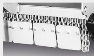
Bolt-on chain's protection plates
