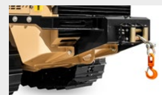
Rear winch with 6 t pulling power
