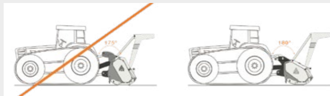
Mulcher designed for tractors with a low profile PTO
