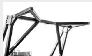
Mechanical push frame guides and pushes material away from carrier
