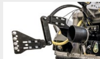
W style self-aligning device between PTO drive shaft/gearbox allows the mulcher to work at several angles without damaging the PTO
