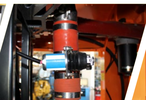
Air shut-off system
