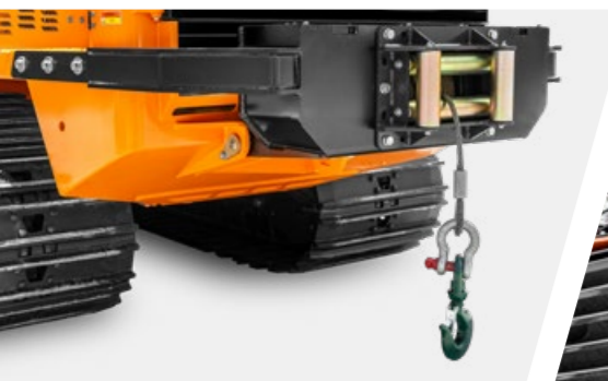
Rear winch with 6-t traction force
