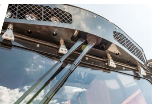
Air window cleaning system
